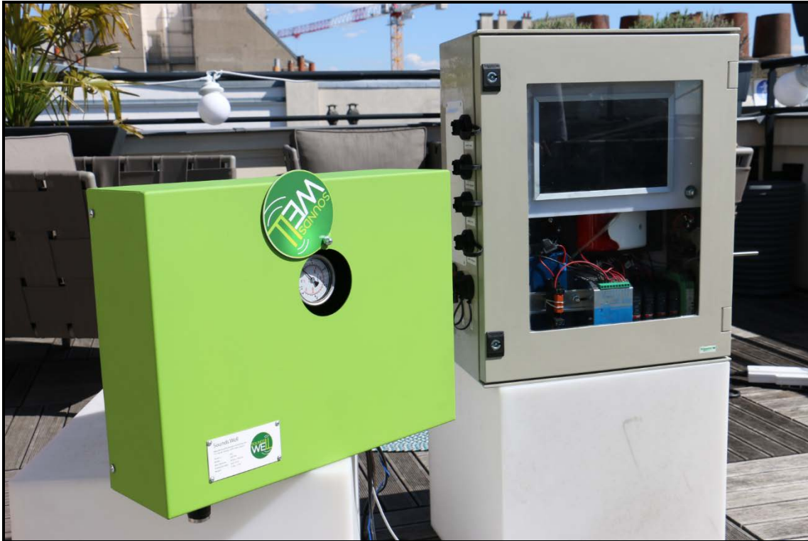
Photo 1 – The Sounds Well system designed for blanket monitoring: a manifold to be plugged to the wellhead (green box on the left) and a data acquisition box (right).
