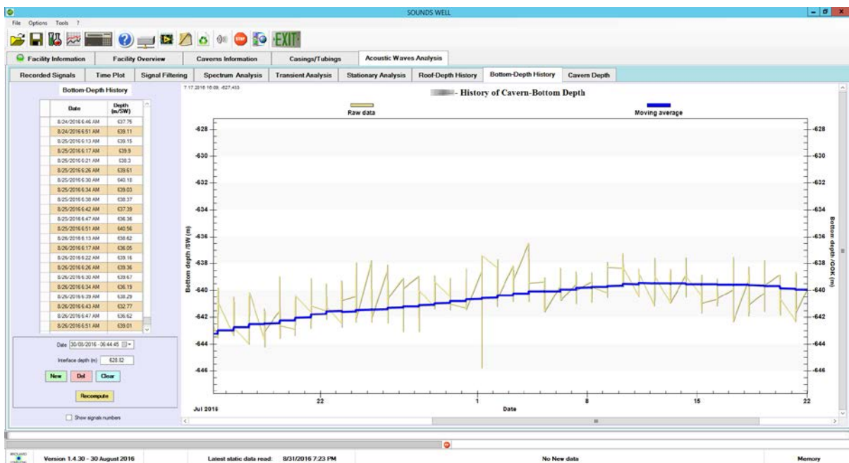
Figure 11 – Sounds Well — Evolution of cavern-bottom depth.
